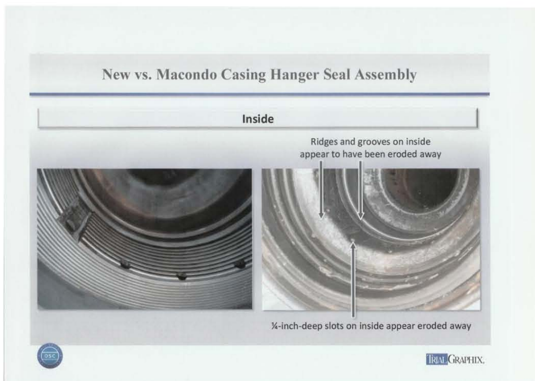
FIGURE 2-9 View inside casing hanger. Source: National Oil Spill Commission, Presentation on the BP Deepwater Horizon Oil Spill and Offshore Drilling, Slides 118-120.
